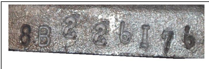
1968 Hamtramck Assembly VIN font reference on an engine block .
