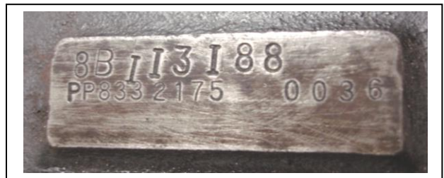
1968 Hamtramck Assembly VIN font reference on a manual the transmission.
