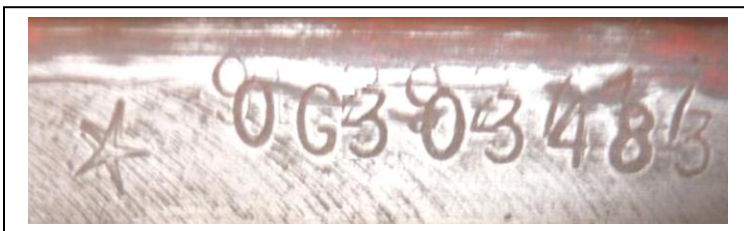
1968 Hamtramck Assembly VIN font reference on an engine block .
